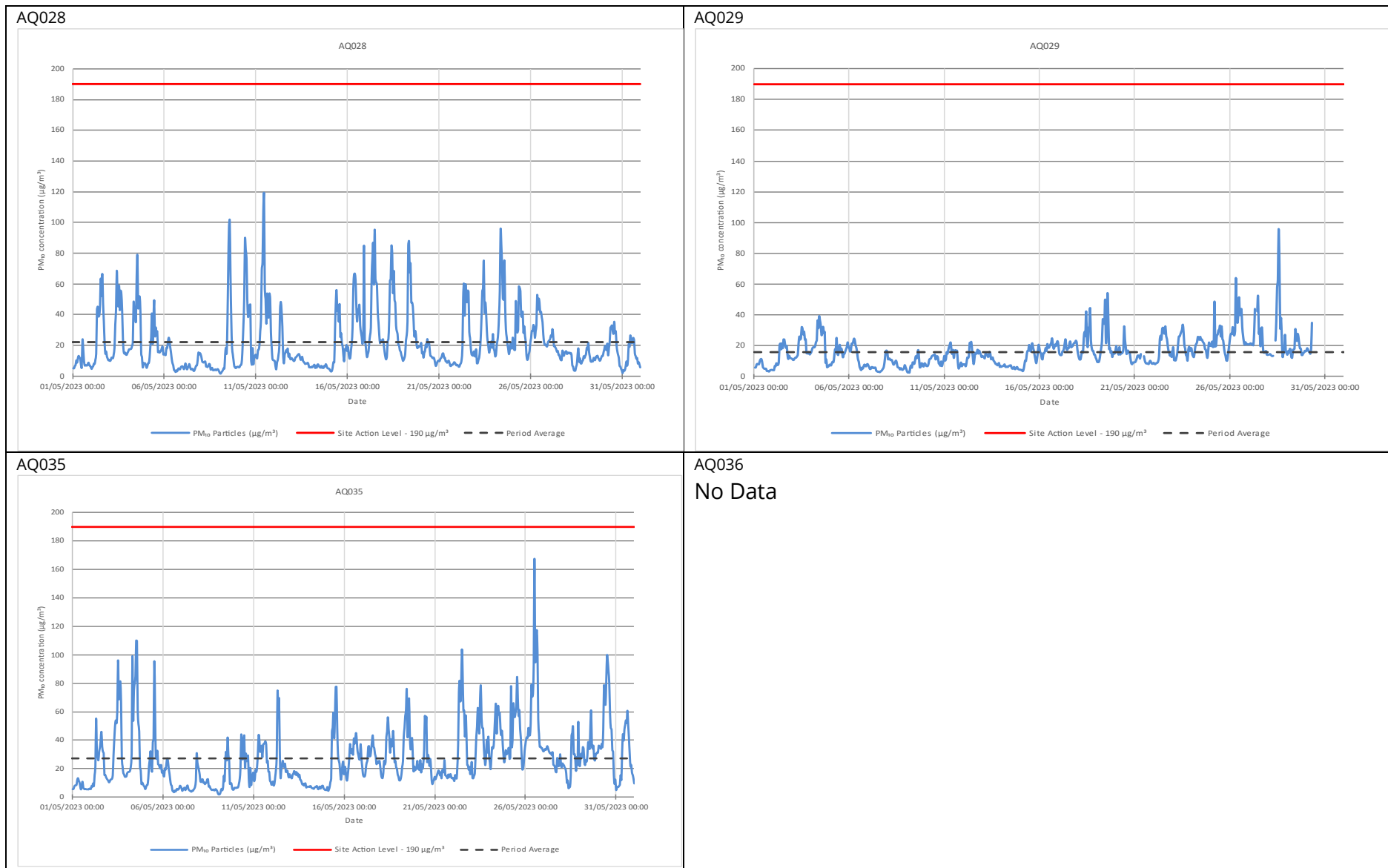
Figure 3: Construction dust 1-hour mean indicative PM 10 concentration for dust monitors
