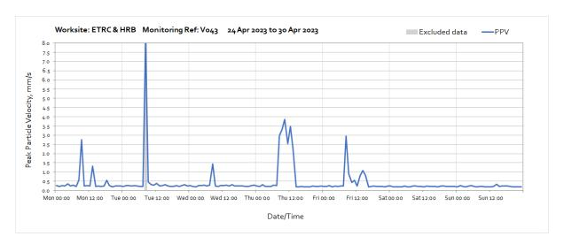
Note: High levels of vibration caused by works close to the monitor. Lower vibration levels anticipated at nearest receptor.
