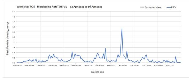
Note: High vibration levels measured between 10:00 and 12:00 on Friday 14<sup>th</sup> April were due to digging of the new haul road and road extension works taking place close to the monitoring station.
