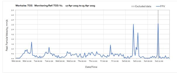
Note: High vibration levels measured at 08:00 and at 13:00 on Saturday 22<sup>nd</sup> April were due to stone compaction works taking place close to the monitoring station.
