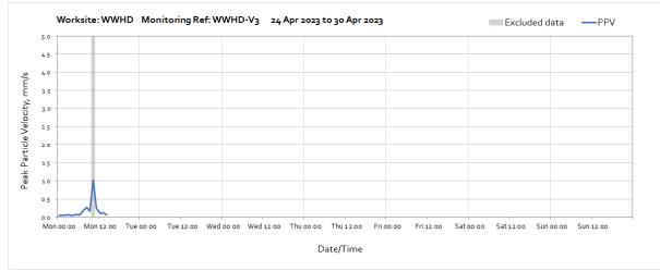
Note: missing data from 15:00 on Monday 24<sup>th</sup> April to the end of the months were due to loss of power at the monitoring station.
