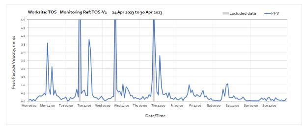
Note: High vibration levels measured across the week were due to excavation, shuttering, concrete pours and stone compaction works taking place close to the monitoring station.
