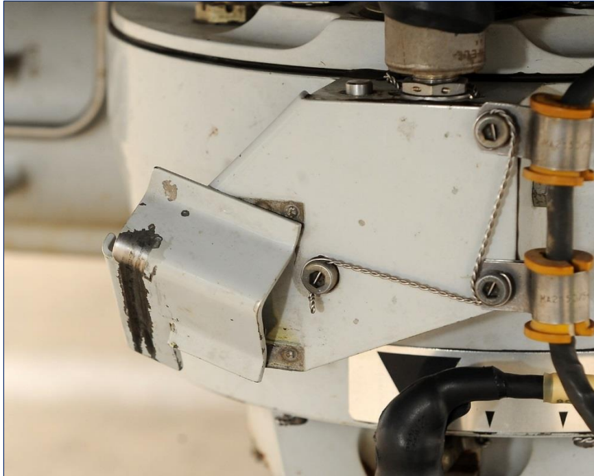
Figure 17 - Deformed Merlin NLG Changeover Valve Striker Plate
