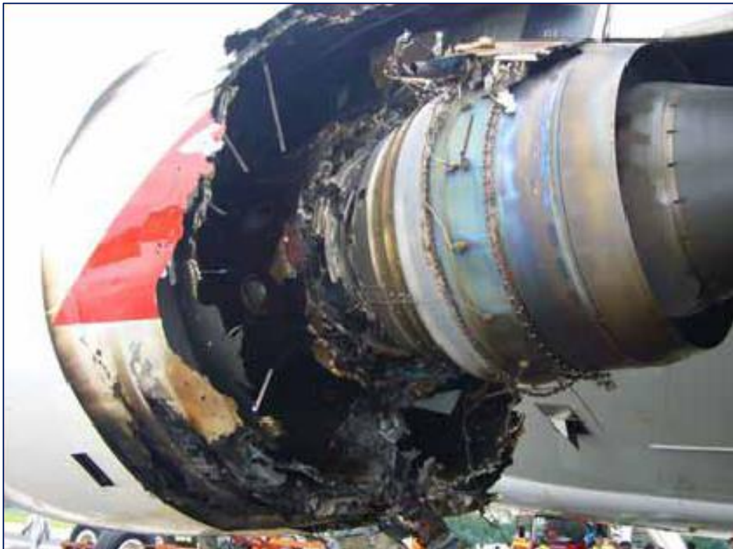
Figure 24 - Trent 900 Uncontained Turbine Disc Damage
