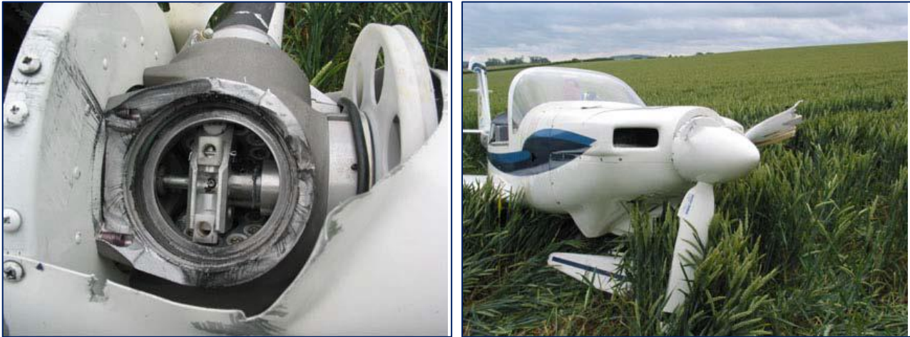
Figure 10 - Propeller hub showing fractured No 1 blade socket
