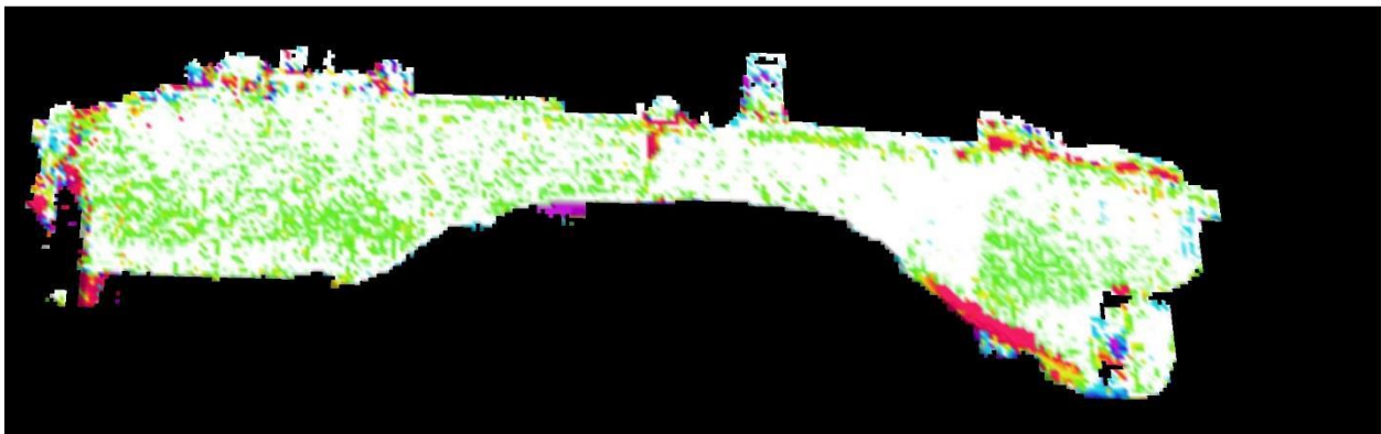
Figure 13 Starboard forward hull surface difference plot between 2017 and 2018 surveys.
