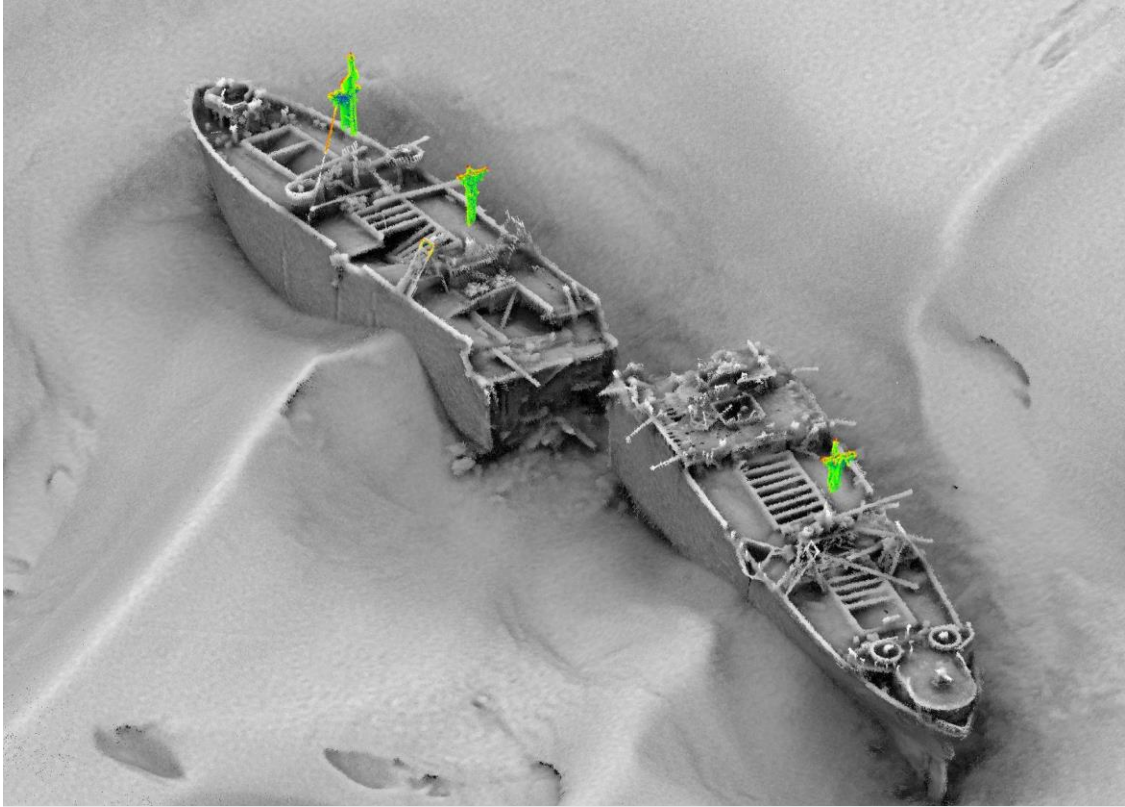
Figure 43 2018 survey Laser scan data points (green to red) integrated with the MBES data.
