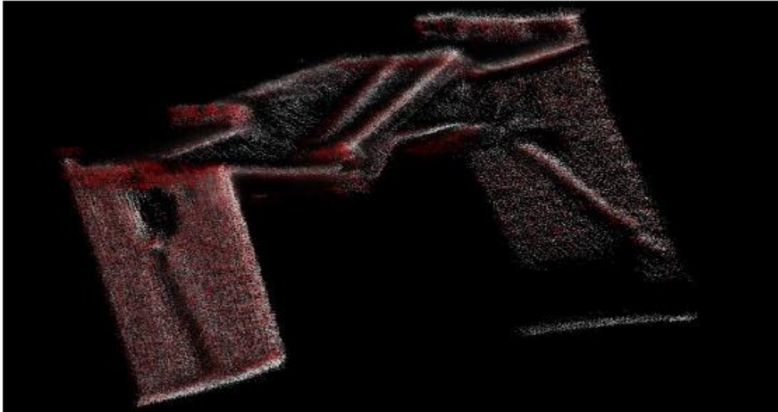
Figure 15: Buckling of the Hull port side inward starboard outward. Red 2021 and Grey 2022 data.
