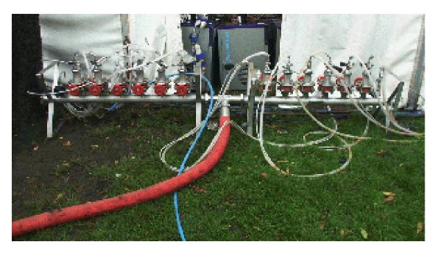
Figure 6 Road Tanker Manifold and coupling devices
