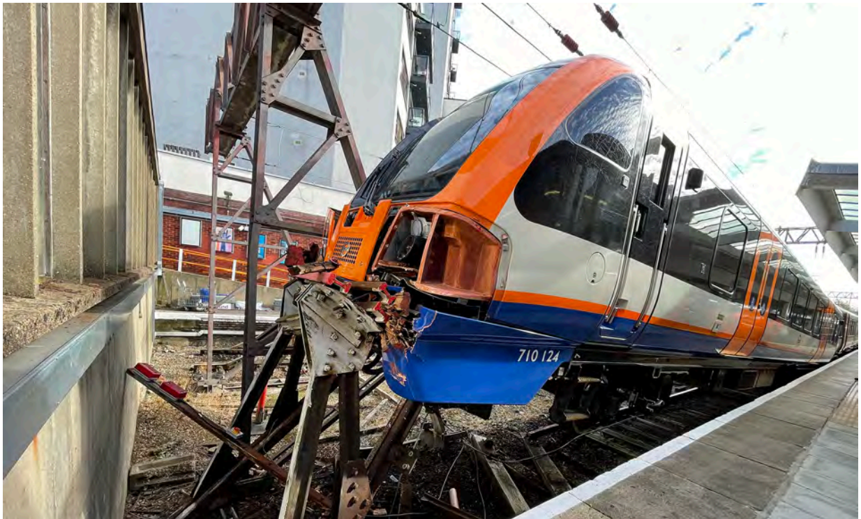
Figure 3: Damage to the front of the train
