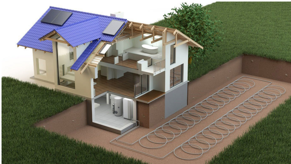
Horizontally sunk ground source heat pump
