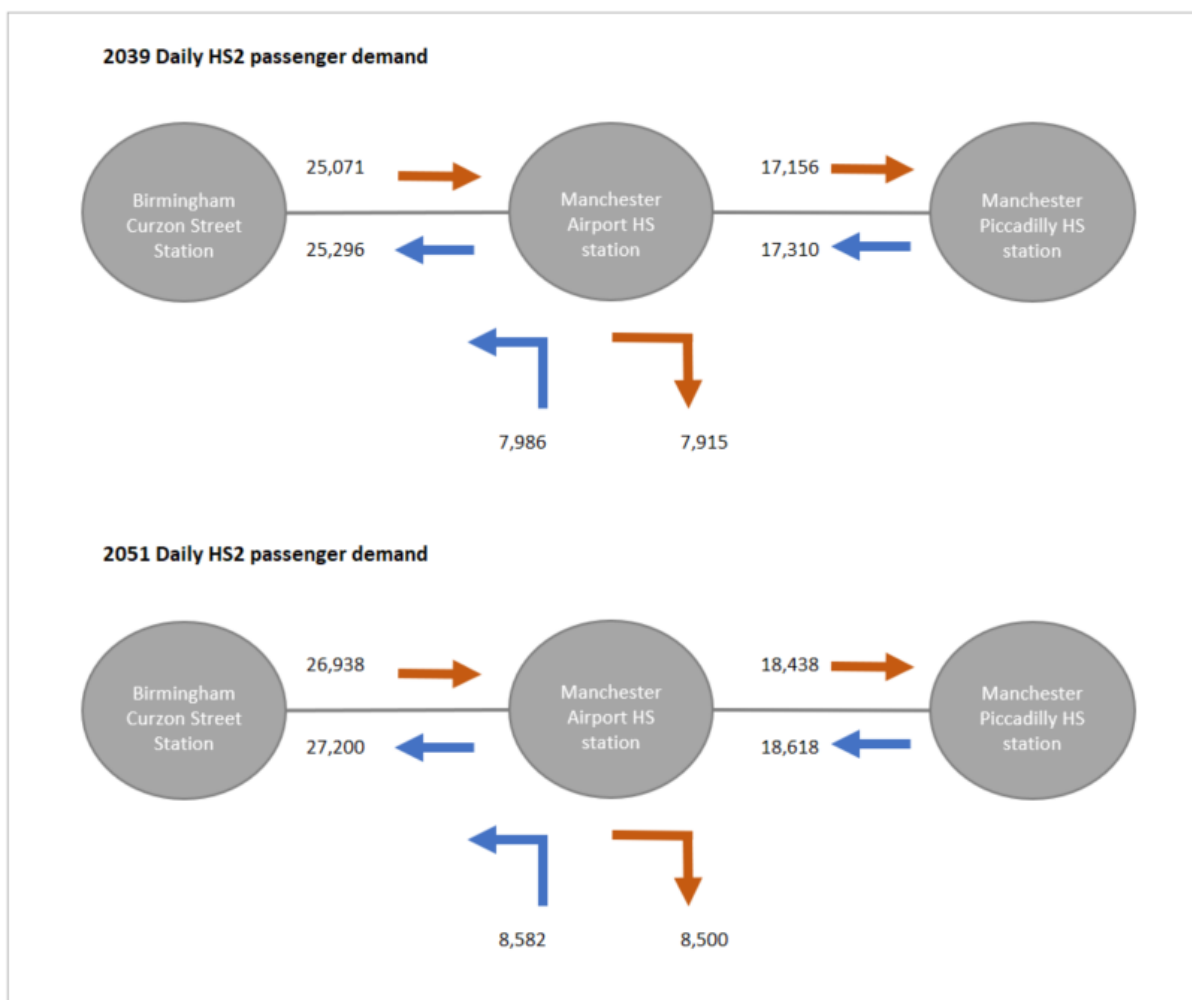
Figure 18-55: AP2 revised scheme daily HS2 demand at Manchester Piccadilly Station and Manchester Airport High Speed station
