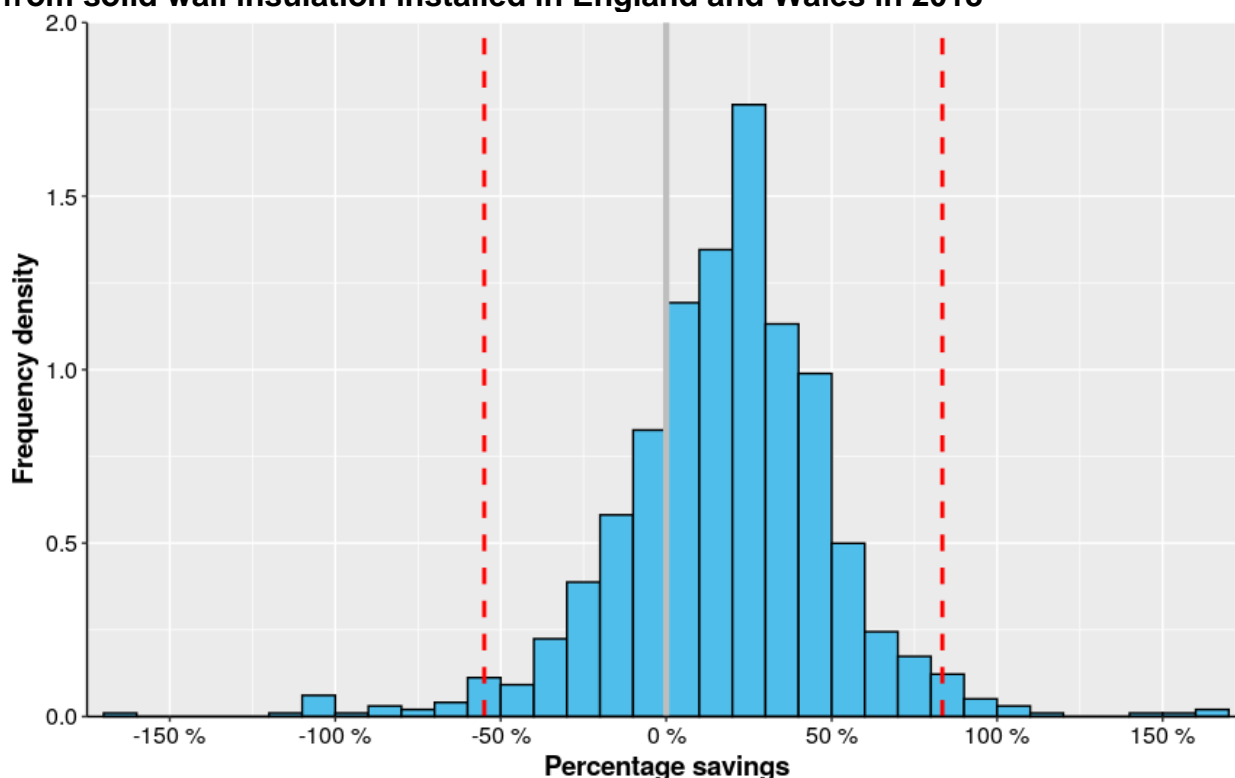
Figure 3.4: The 95 per cent filtering boundary for the gas percentage savings in 2019 from solid wall insulation installed in England and Wales in 2018
