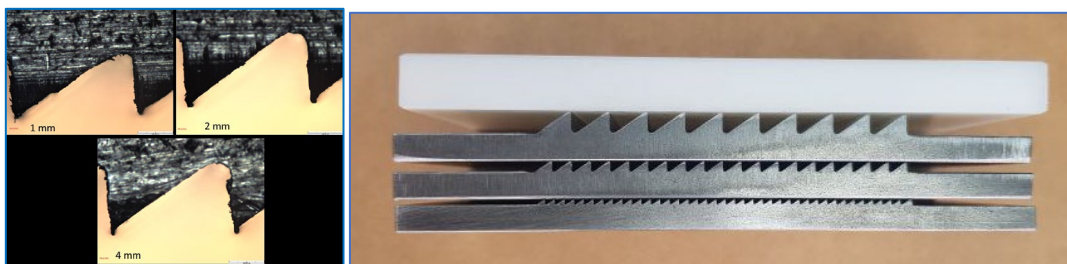
Figure 3-1 - Test Coupons used for Tooth Penetration Tests with NPL Tip Profiling
