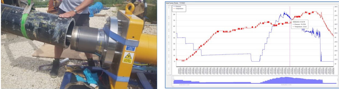
Figure 3-3 - Test swaging trial of 12inch diameter pipe section with pressure test data
