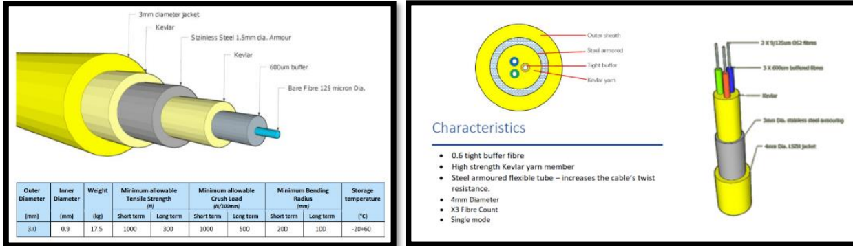
Figure 4-4: Jacketed Micro Armoured Stainless Steel SMF G 652 Fibre (i) 3mm, single core, (ii) 4mm 3 core
