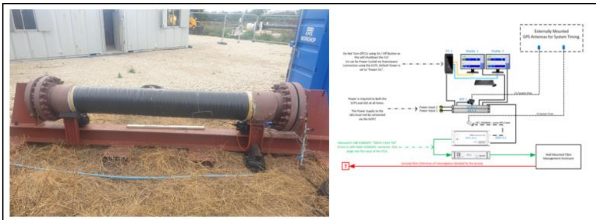
Figure 8-2: MASiP Pipe 11 setup for the fatigue cycling tests.
