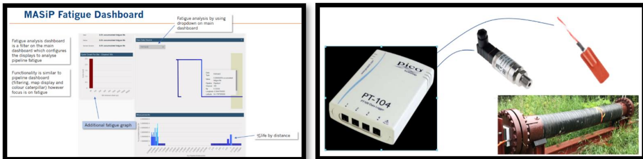
Figure 5-3: Fatigue analysis and alerting dashboard and pressure and temperature transducer link
