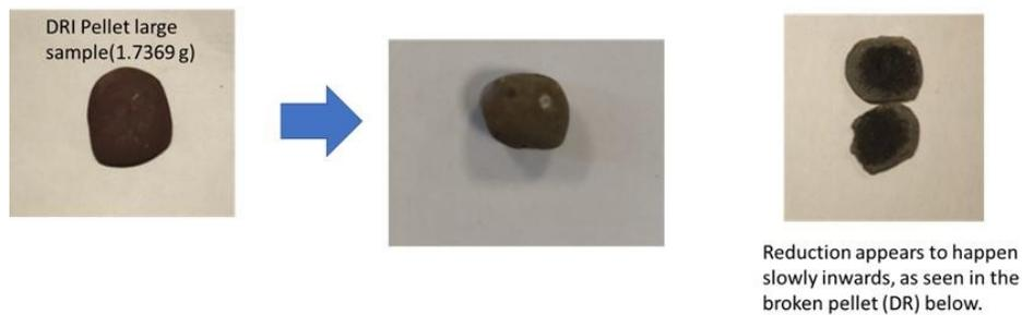
FIG. 16: PROGRESSIVE REDUCTION FROM SURFACE TO CORE IN LARGE DR PELLETT
