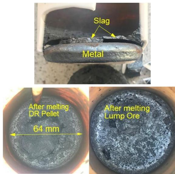
FIG. 25: MELT 4 TEMPERATURE PROFILE & PRODUCTS
