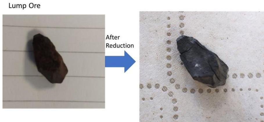
FIG. 14: LUMP ORE PARTICLE: AS RECEIVED AND AFTER REDUCTION
