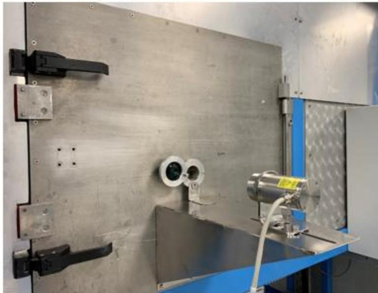
FIG. 22: PHOTOGRAPH OF C-TECH INNOVATION HYBRID KILN DOOR WITH EXTERNALLY MOUNTED PYROMETER
