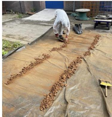
FIG. 1: DIVIDING LARGE LUMP ORE SAMPLE INTO REPRESENTATIVE SUBSAMPLES
