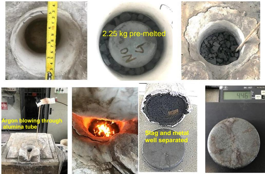
FIG. 27: MELT 9; 100 KW INDUCTION FURNACE, 6 KG LUMP ORE
