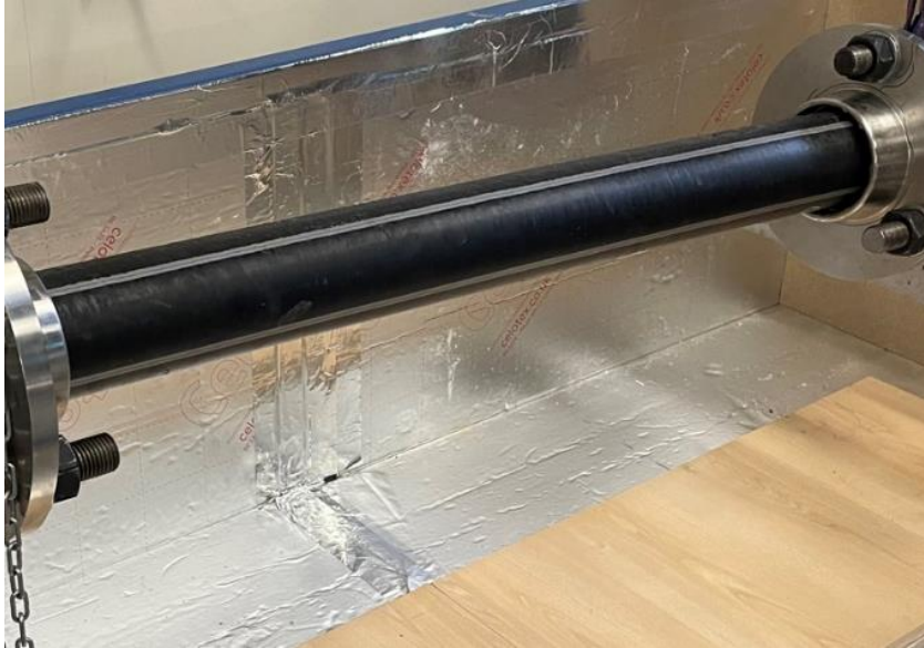
Figure 24 Pipe samples prepared for burst testing
