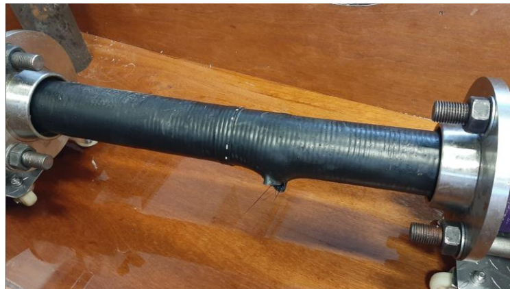
Figure 27 Failure in prototype pipe sample after burst test
