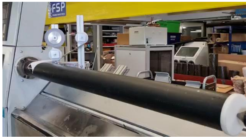
Figure 16 Early trials using filament winding machine for pipe manufacture
