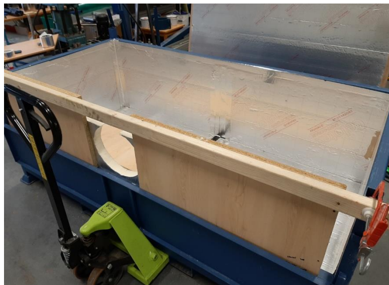
Figure 23 Chamber for burst tests
