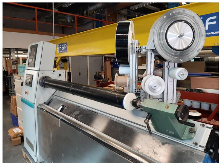
Figure 17 Final version of filament winding machine for pipe manufacture
