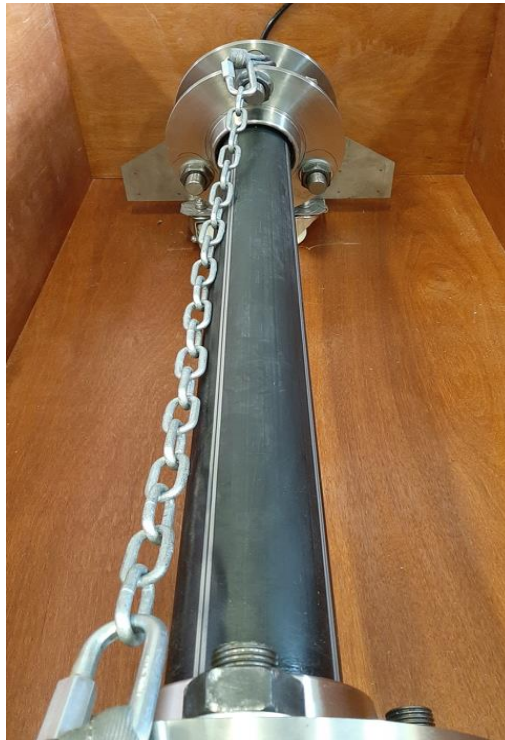
Figure 25 Pipe sample prepared for burst testing
