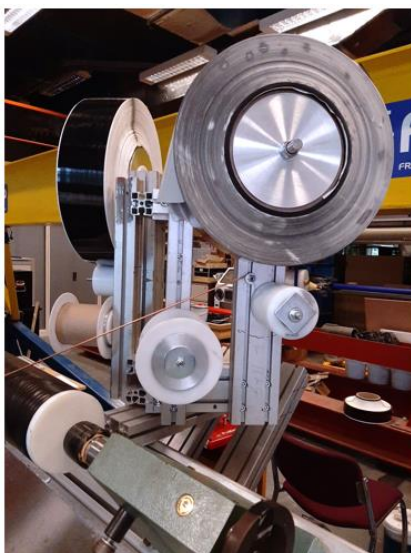
Figure 16 Early trials using filament winding machine for pipe manufacture
