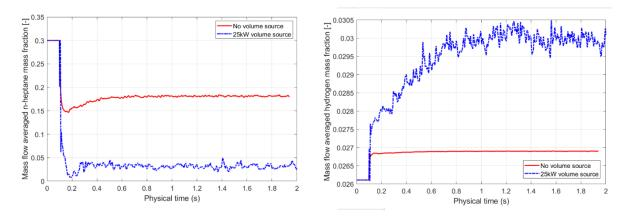
Figure 2: The distribution of key mass flow averaged quantities across all syngas flow outlets with and without the triboplasma volume source: n-heptane mass fraction, which represented tars in the simulation (left) and hydrogen mass fraction (right).
