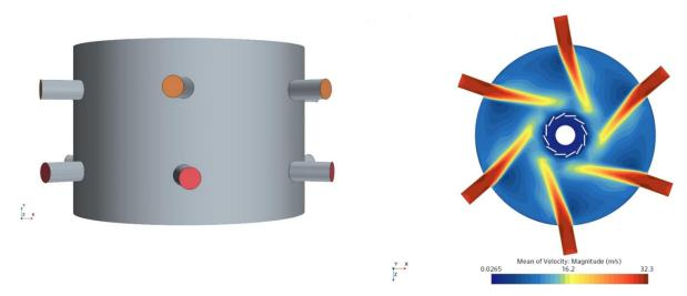
Figure 1: Schematic of reformer vessel used in the full-scale reacting flow calculations, where inlets are highlighted in red and outlets are highlighted in orange (left) and the CFD solution of in the reformer inlet plane coloured by mean velocity magnitude (right).
