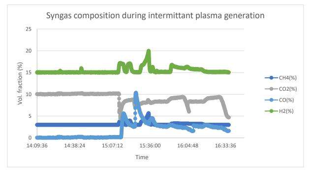
Figure 3: Syngas analysis from tests at UCL, in which a gas mixture of H2, CO2, Steam, CH4 and vaporised C12 hydrocarbons are exposed to intermittent plasma discharges
