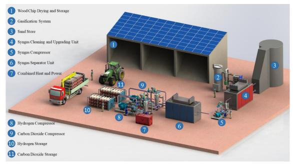
Figure 6: Digital Representation of the Layout for NEW<sub>2</sub>H<sub>2</sub> Concept 3
