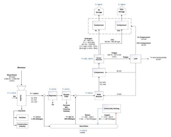
Figure 7: Heat and Mass Balance Diagram for the Proposed NEW2H2 Concept 3 Installation
