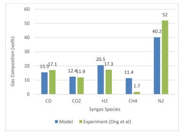
Figure 11: Validation Comparison Between the Developed Model and the Experimental Data for Wood Chips
