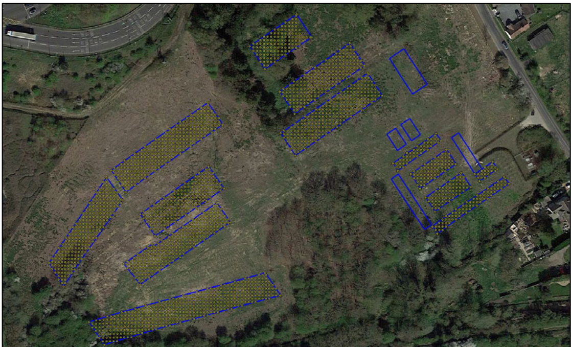
Figure 22 Reflecting areas 8 (yellow radial icons) – Pager Power modelling results for ATC Tower
