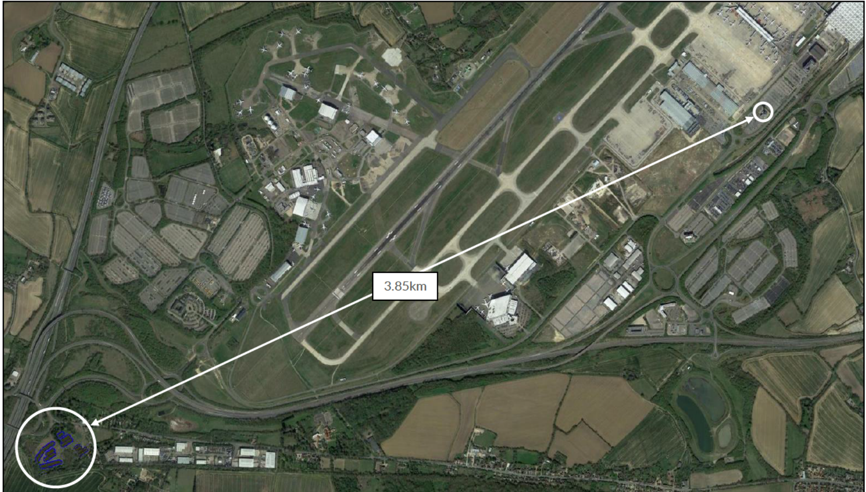
Figure 16 Reflecting areas relative to the ATC Tower
