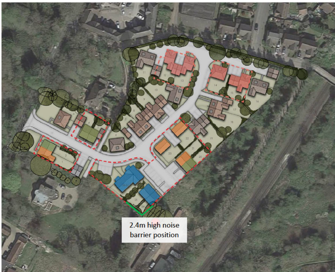
FIGURE 2 – SITE PLAN SHOWING ACOUSTIC FENCE LOCATION
