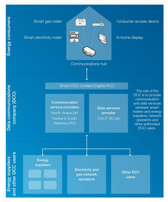
Figure 4: Overview of the smart metering system
