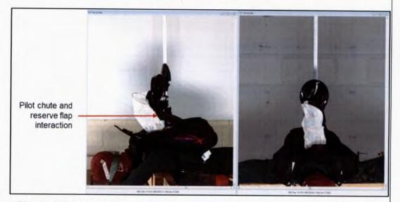
Figure 1.4.24 – HSDV test R17 in a total malfunction configuration, RPC material interaction.
