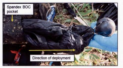
Figure 1.4.12 – Main pilot chute being extracted by TVP.
