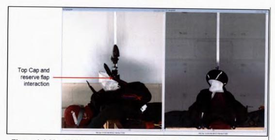
Figure 1.4.23 – HSDV test R17 in a total malfunction configuration, top cap interaction.
