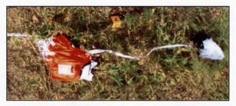
Figure 1.4.6 – Disturbed reserve parachute, free-bag and pilot chute.
