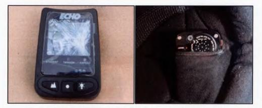
Figure 1.4.9 – Sgt Fisk's damaged Larsen & Brusgaard ECHO (left) and as stowed in helmet pocket (right).
