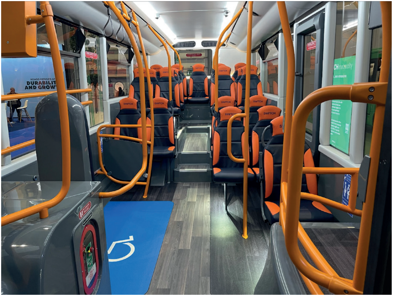
Figure 5 The inside of a bus showing the wheelchair space, handrails and handholds, seats, and steps (DfT)
