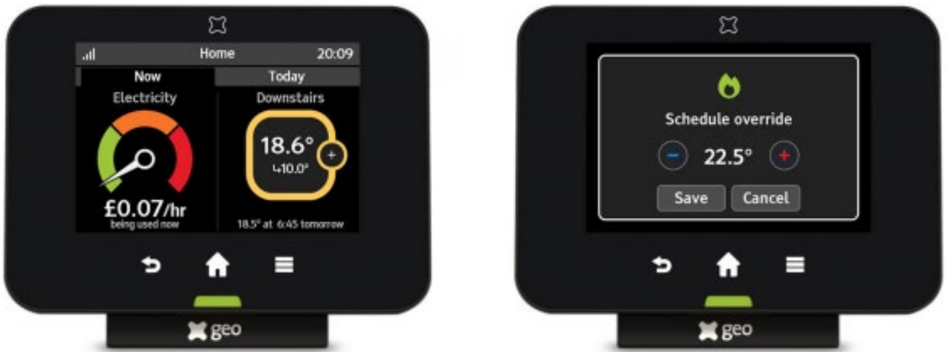
Figure 1: Examples of information presented through the SENS-ST smart thermostat. The device combined smart meter data (see left) and heating data
