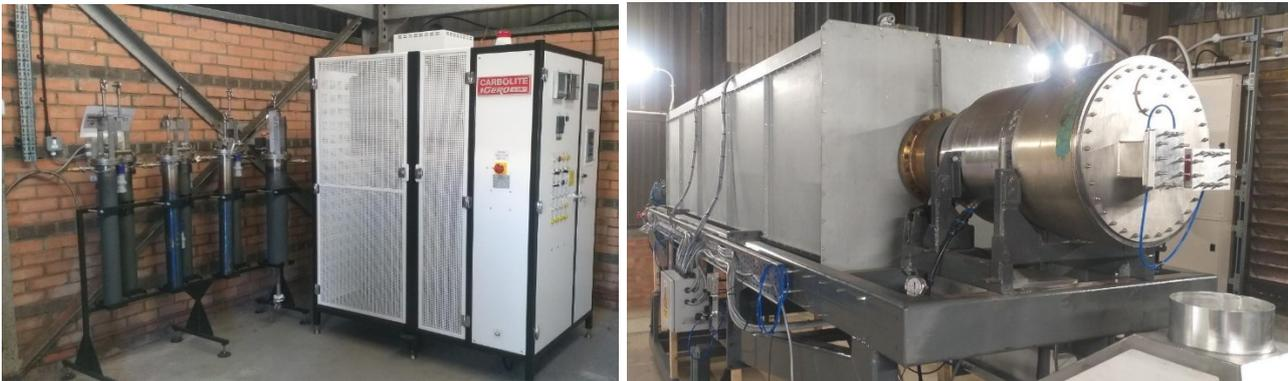
Figure 9. Left: iron ore reducability rig. Right: rotary reduction furnace at the MPI.
