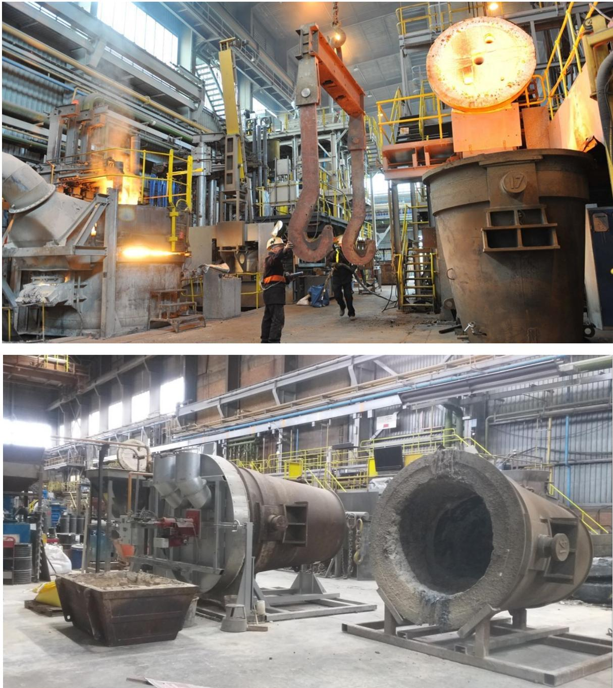
Figure 10. Steel ladles and preheater stations in the MPI Normanton Pilot Plant: (top) 7-ton steelmaking ladle at a preheater station (foreground RHS) ready to receive tapped steel
