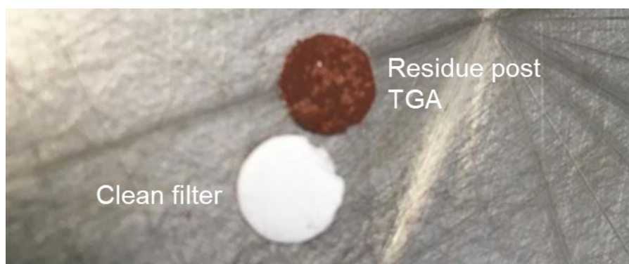
Figure 5-33: Residual material on brake PG-42 PM filter section post TGA analysis
