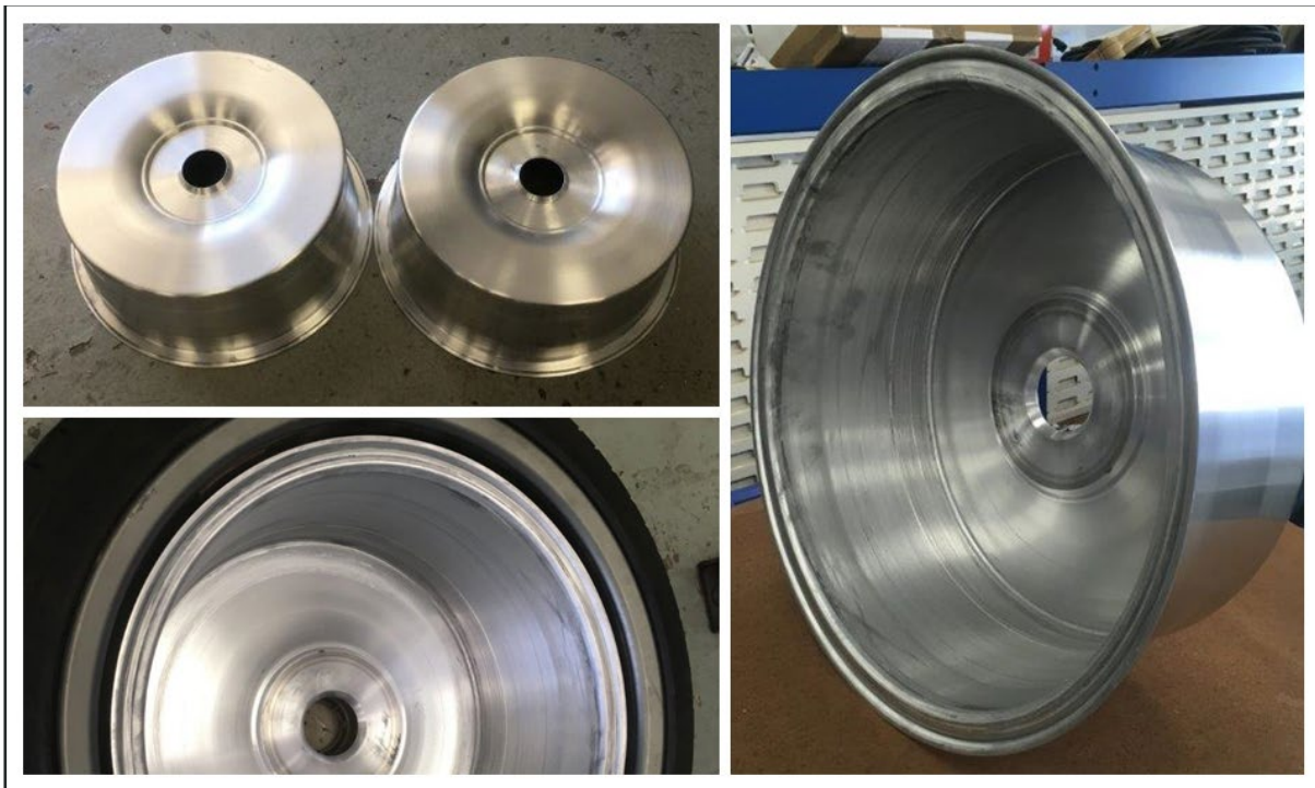
Figure 5-8: Single piece spun aluminium enclosure for designs B and C
