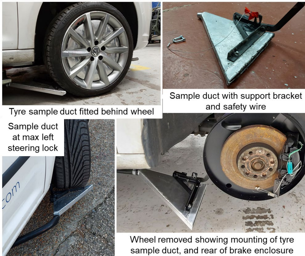
Figure 5-12: Tyre particulate sample duct
