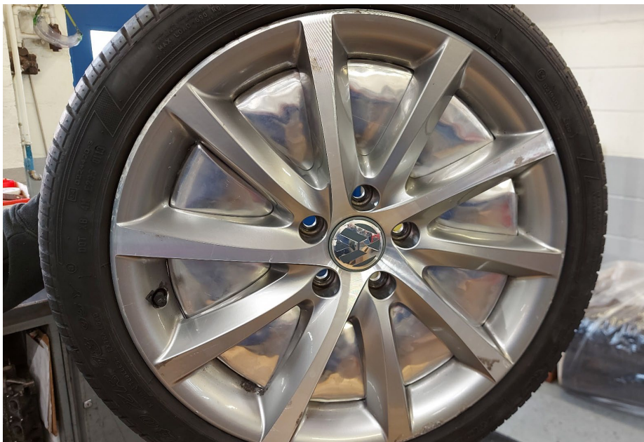
Figure 5-5: Brake enclosure design option A: Wheel face sealed with an aluminium disc
