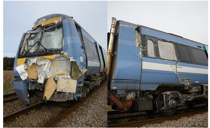
Damage to the train involved in the collision at Hockham Road in 2016.
