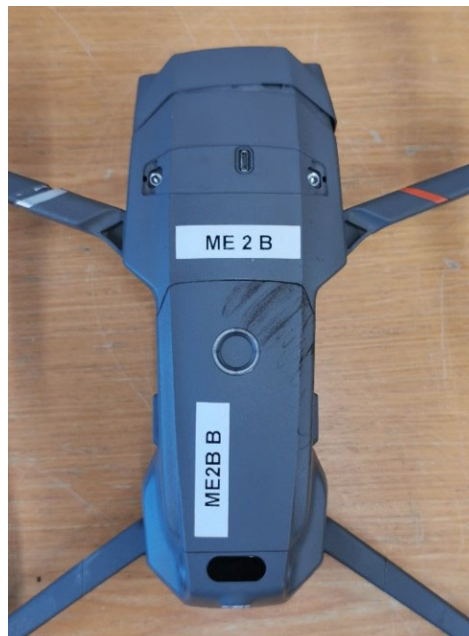
Figure 4 Accident battery re-installed in accident Mavic
