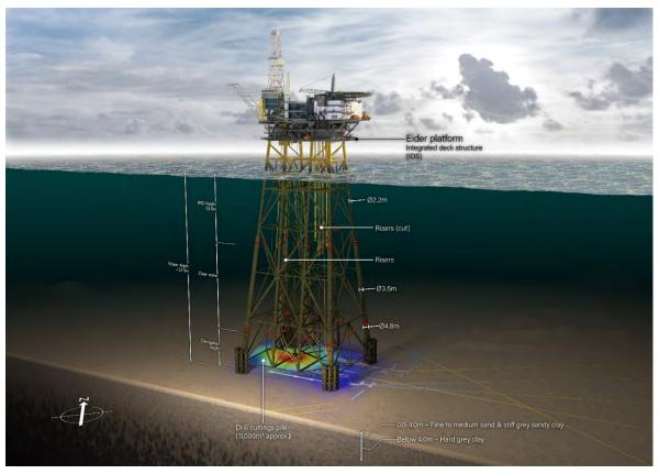
Figure 2-2 Eider decommissioning schematic
