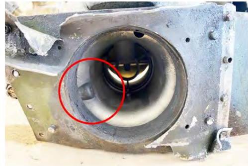
Missing accelerator pump discharge tube from G-BBSA carburettor
