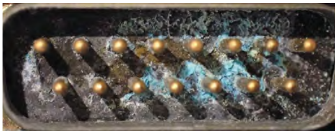
Contamination and corrosion on the audio warning unit connector
