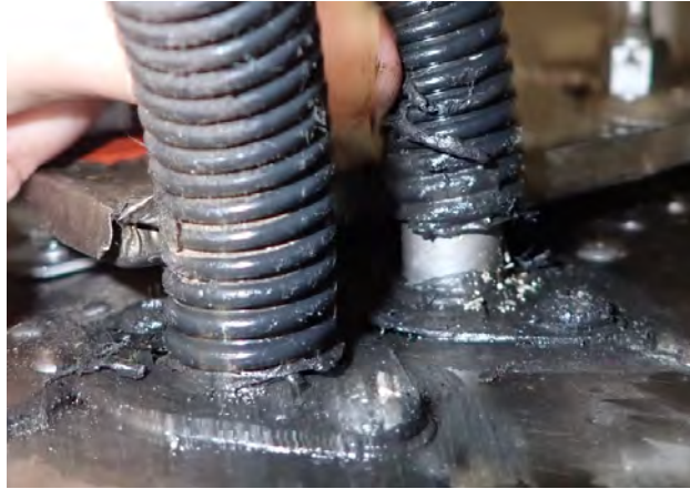
Right engine ignitor cable sheath easily moved away from deck
