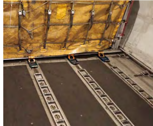
ULD rails and locking mechanisms
