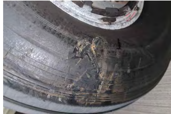
Damage to one of the landing gear tyres
