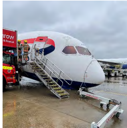
View of the right side of the aircraft following NLG retraction
