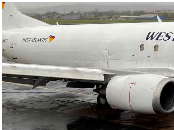
Photograph looking aft showing distortion of the rear fuselage and rippling in the skin
