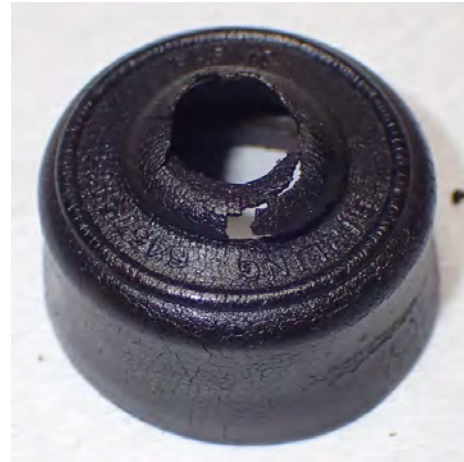
A dust seal from one master cylinder showing degraded condition
