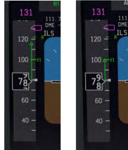
PFD Speed Tape trend arrow (left image with 89% N 1 , right image with 70% N 1 ) (Images captured on a simulator)
