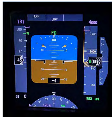
PFD prior to starting the takeoff (image captured in a simulator)
