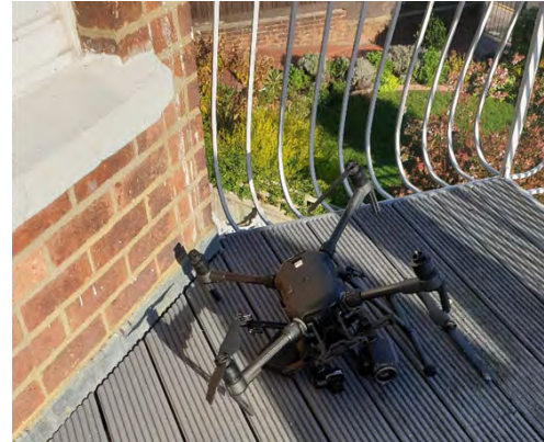
Damage to UA
