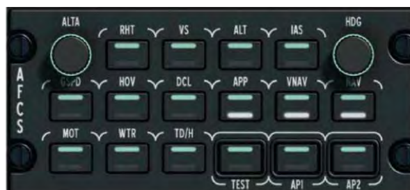
Autopilot Control Panel
