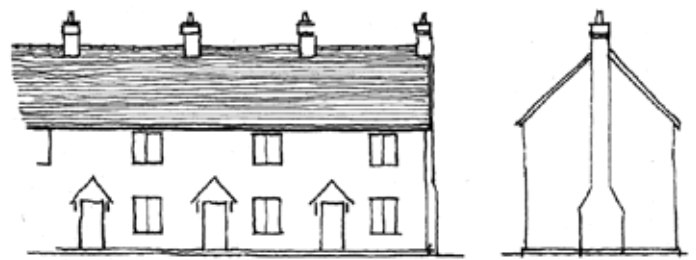
Front elevation with minimum openings. Illusion created of larger houses: door opening could control windows to either side
