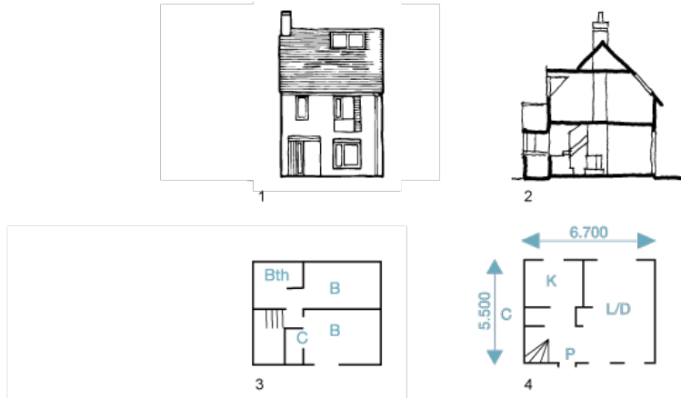
1. Front elevation 2. Section 3. First-floor 4. Ground-floor
