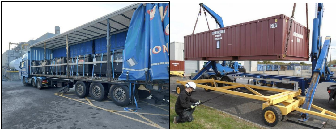
Photographs 3 & 4: LLW Combustible wheelie-bin shipment and half-height ISO shipment of metallic waste
