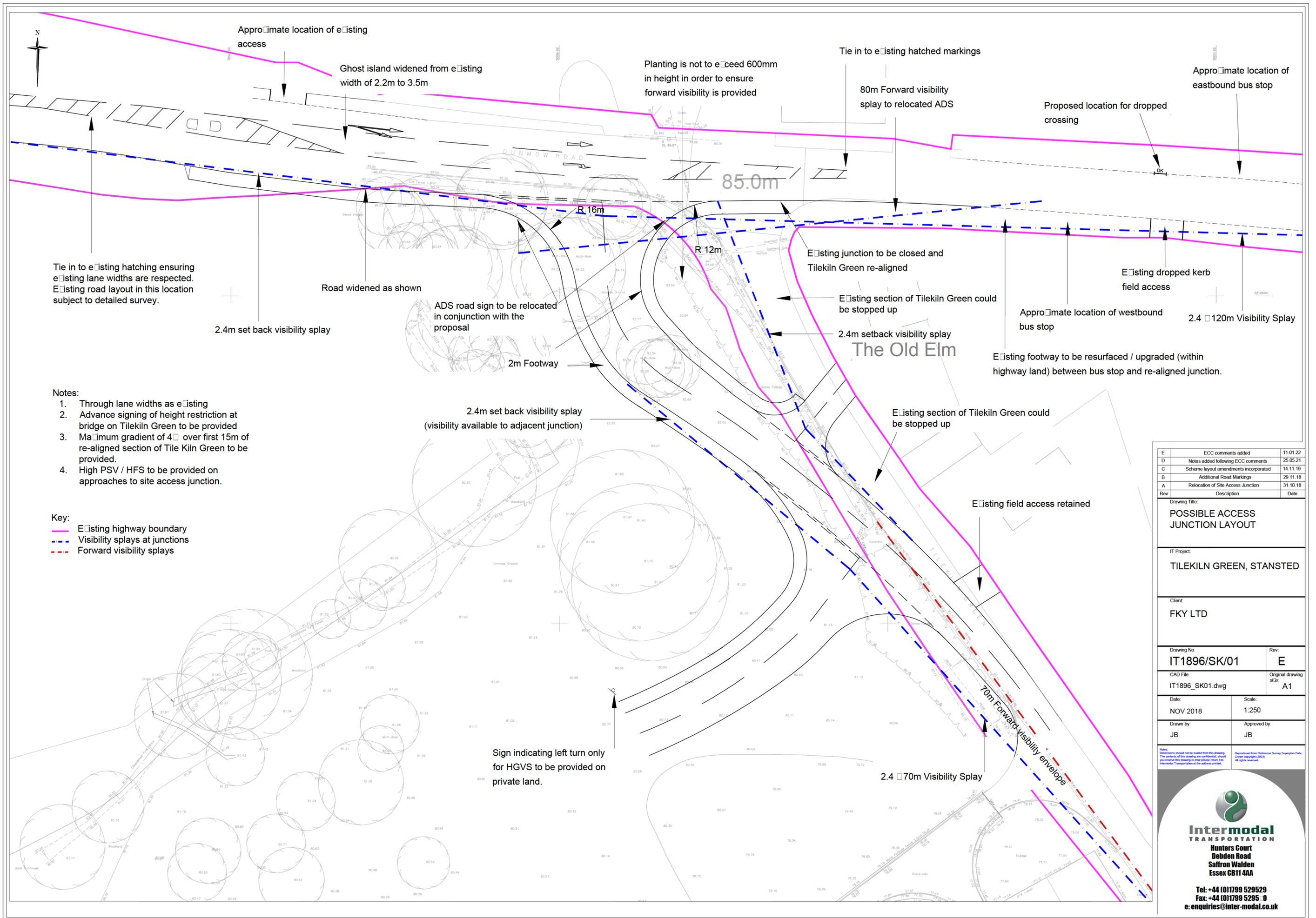
Tie in to existing hatching ensuring existing lane widths are respected. Existing road layout in this location subject to detailed survey.
