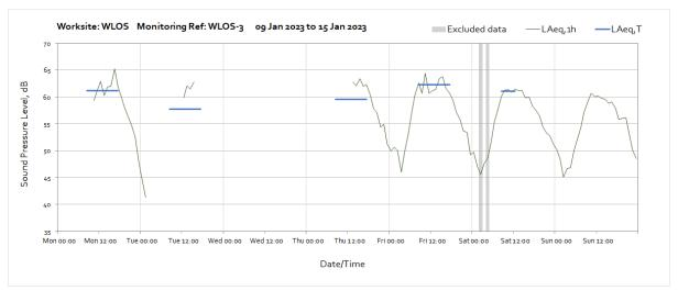
Note: Missing data throughout the week was due to loss of power to the battery from the solar panels. The batteries were replaced on Thursday 12<sup>th</sup> January.
