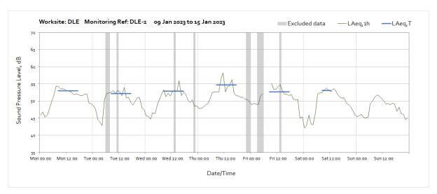
Note: Missing data between 06:00 and 09:00 on Friday 13<sup>th</sup> January was due system malfunction leading to loss of power supply to the monitor.
