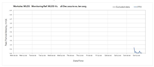
Note: Missing data throughout the week was due to damage to the solar panel resulting loss of power to the monitor. Panel batteries replaced on Tuesday 17<sup>th</sup> January and solar panel replaced on Tuesday 24<sup>th</sup> January.
