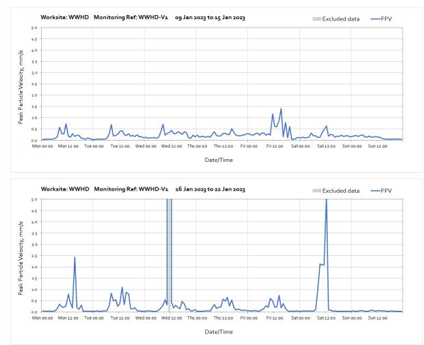
Note: High vibration levels measured between 09:00 and 12:00 were due to movement of plant on haul road close to monitoring station.
