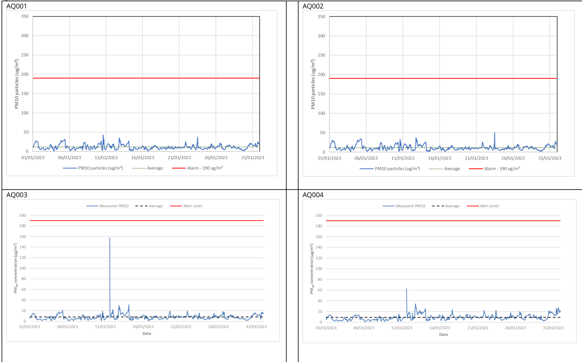
Figure 4: Construction dust 1-hour mean indicative PM 10 concentration for dust monitors
