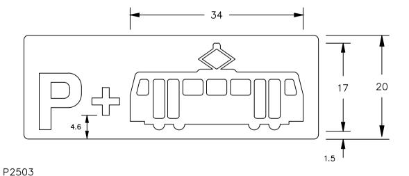
NOTES: 1. Symbol details are given on drawings S 25 sheet 1, S 26, S 38, S 39 and S 43.
