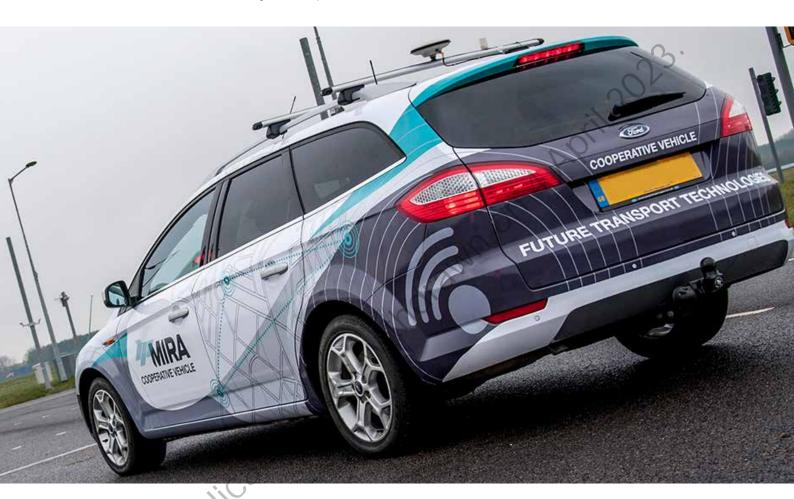
In some cases, the sensors use lasers to measure the distance to objects. These are used to build up a 3D map of the area.
