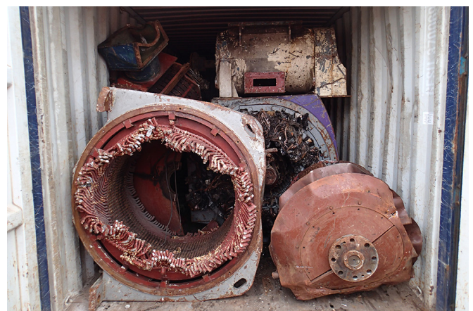
An example of asymmetric loading of heavy scrap electrical machinery.
