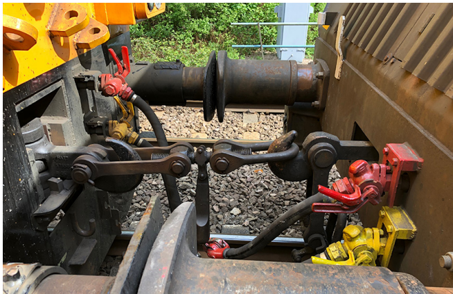
Positions of brake pipe valves on locomotive involved in the SPADs at Crofton.
