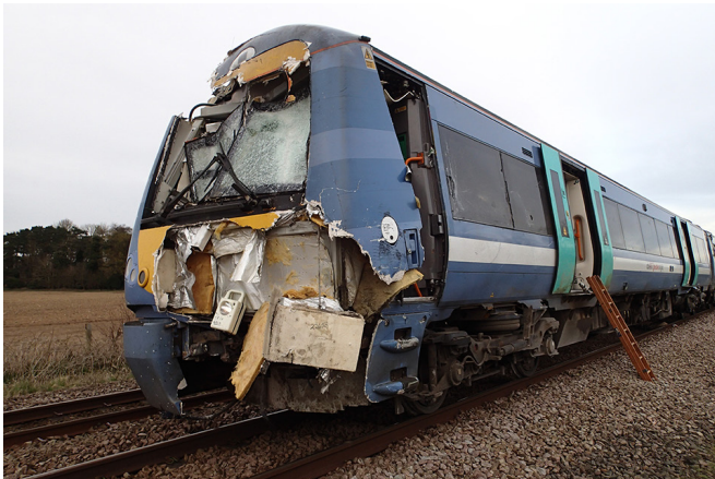
Damage to the train involved in the collision at Hockham Road in 2016.
