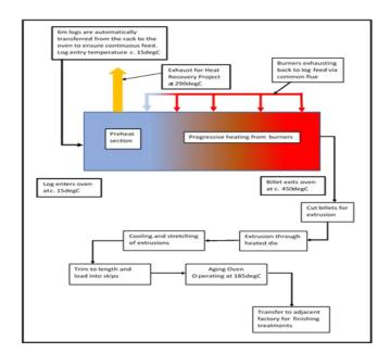
Picture on the left shows one of the log ovens, where aluminium is heated up to 450°C Picture on the right shows a Flow Diagram of the process.
