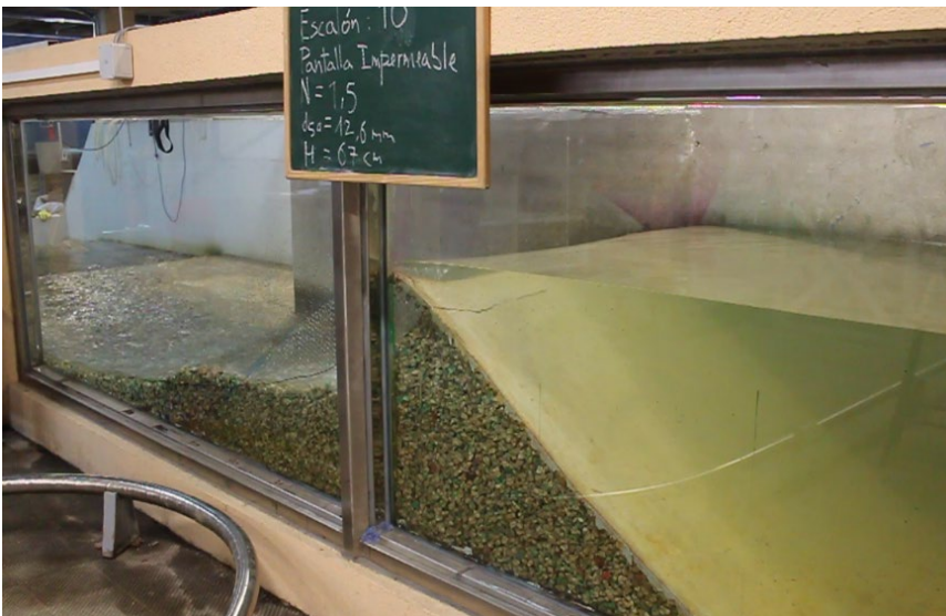
Figure 16 - Image of flow over thin protection layer leading to slumping or porous rockfill and subsequent cracking and failure of protection layer in rockfill erosion tests
