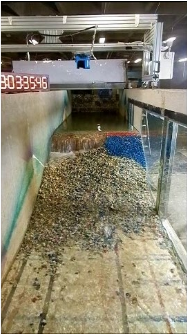
Figure 15 - Image of flow over thin protection layer leading to slumping or porous rockfill in rockfill erosion tests
