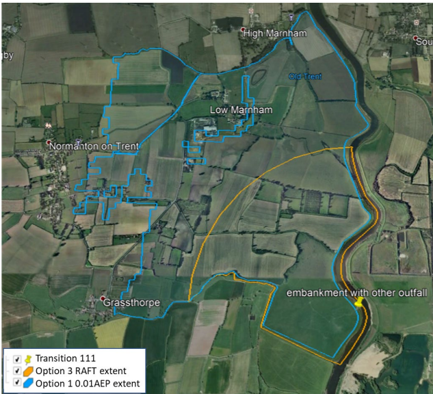
Figure 3-2 Comparison of flood extents for Transition 111
