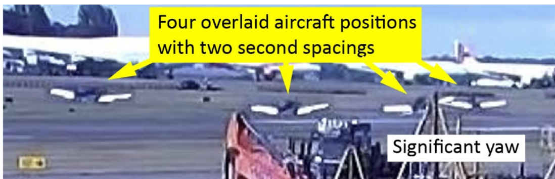
Figure 6 Four cropped CCTV images, two seconds apart, overlaid to show change in heading
