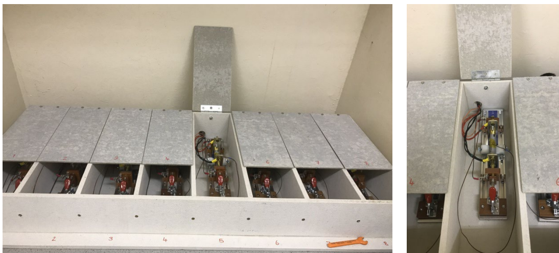
Figure 4 Custom built cell holding enclosure (1 cell per section)
