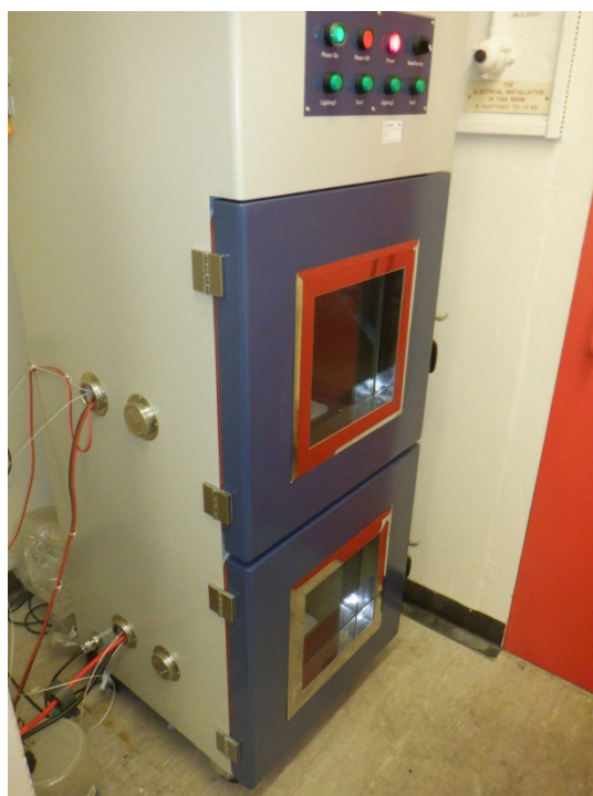
Figure 25 Ventilated test enclosure within blast chamber
