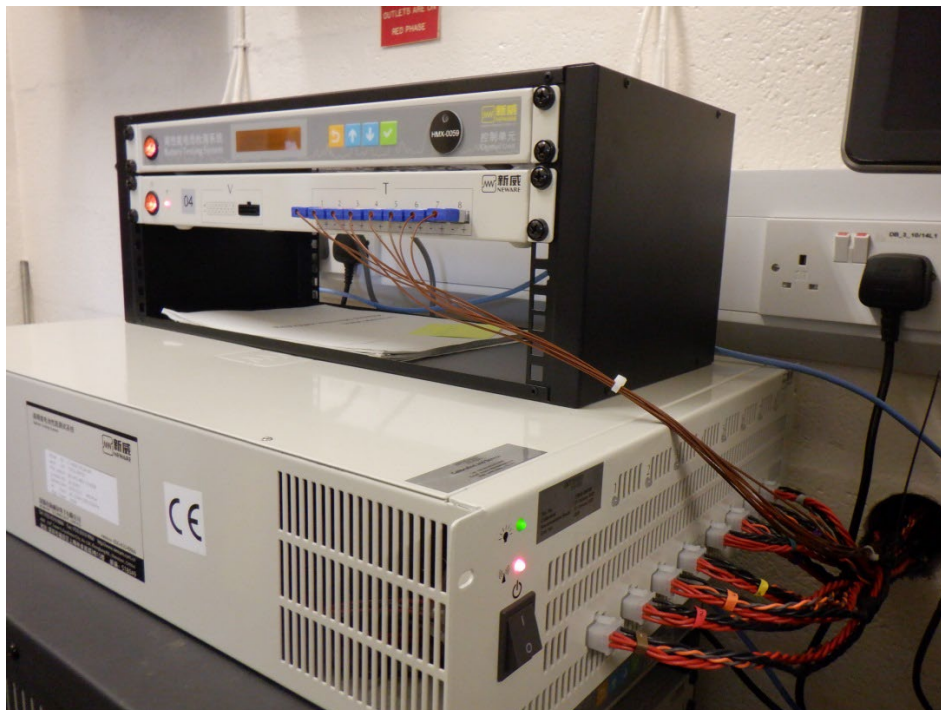
Figure 3 Cell cycler- Control and temperature unit on top, power unit (beige) showing power cable bundle going into blast cell
