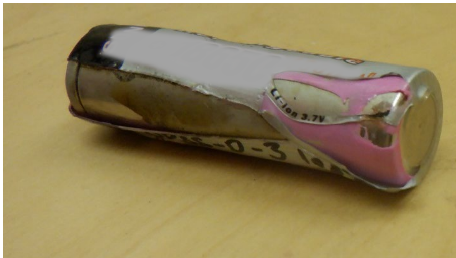
Figure 35 Cell D post-test
