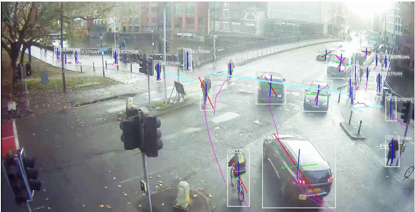
Figure 1 Visualisation of sensors classifying different road users alongside traffic lights which can be connected for autonomous operation, VivaCity
