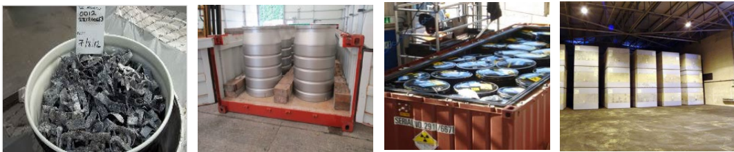
Left to right, Fuel element debris, steel drums of encapsulated waste, drums of plutonium contaminated waste, boxes of waste from Windscale AGR.
