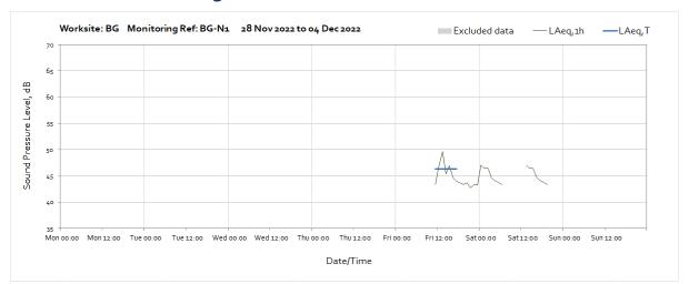
Note: Missing sections of data throughout the week were due to power supply issues as the monitor battery was not receiving sufficient charge.
