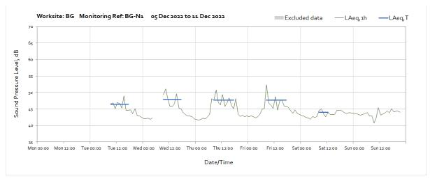
Note: Missing sections of data throughout the week were due to power supply issues as the monitor battery was not receiving sufficient charge.
