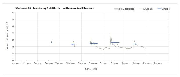
Note: Missing sections of data throughout the week were due to power supply issues as the monitor battery was not receiving sufficient charge. Following the persistent issues the monitor was later retrieved for repair with a suspected hardware issue.
