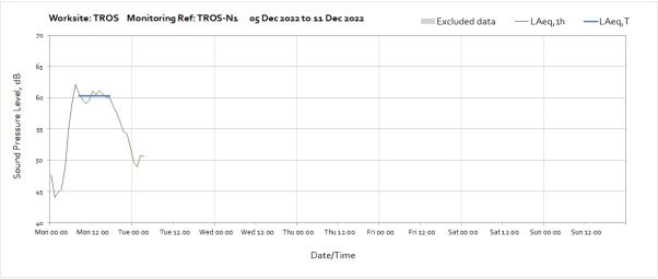
Note: Missing data from 04:00 on Tuesday  $6^{th}$  December till end of the month was due to loss of power to the monitor as solar battery supply was not able to charge. The batteries were replaced on  $22^{nd}$  December.
