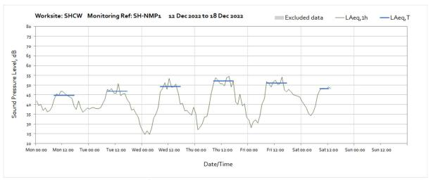
Note: Missing data from 14:00 on 17<sup>th</sup> December until month end was due to battery charging problem, solar enclosure has been retrieved for repair.
