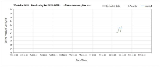
Note: Missing data throughout the week of 28<sup>th</sup> November was due to depleted monitor battery, battery cable has now been replaced.
