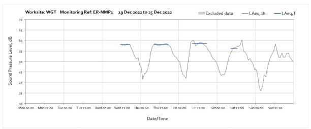
Note: Missing data from 20:00 on 15<sup>th</sup> December until 11:00 on 21<sup>st</sup> December was due to depleted monitor battery.
